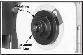
Figure 22. Wheel retaining nut.
